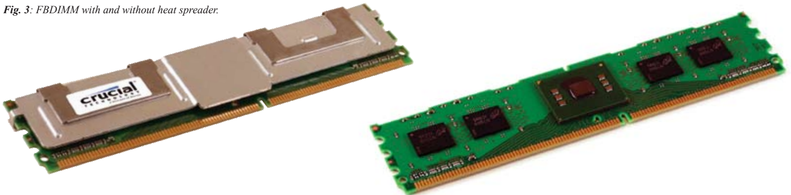
Fig. 3: FBDIMM with and without heat spreader.
